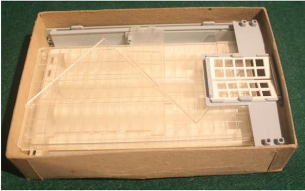
Photo 7: place the front wall, face down, into the box with the wall to the outer edge of the box.
