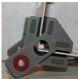
**Magnetic Snap & Glue Set** - This set is also handy for holding pieces at right angles for gluing. These can be placed anywhere along a the pieces being glued as long as they are at right angles
